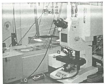
Fig. 1. HYPERION 3000 FPA imaging IR-microscope adapted to the IFS 66v/S FT-IR spectrometer at the ANKA IR-beamline.
